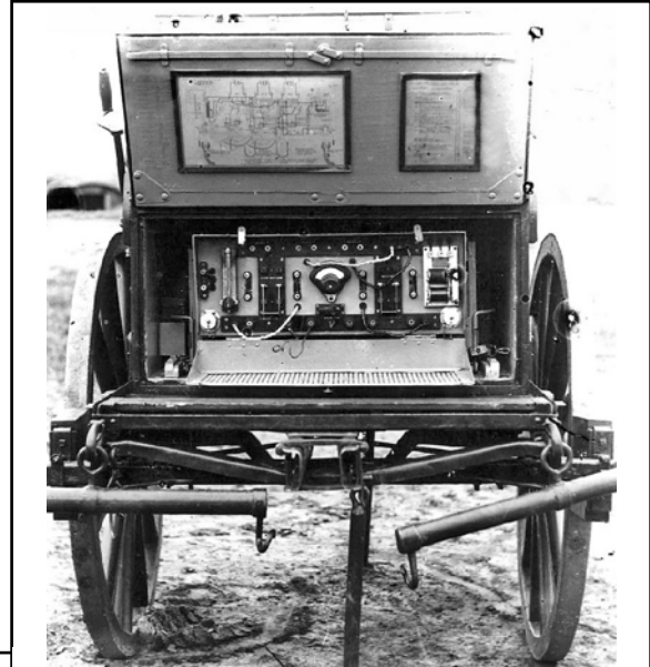
RKA accumulator charging panel fitted under the driver's seats at the front side of the limber.
