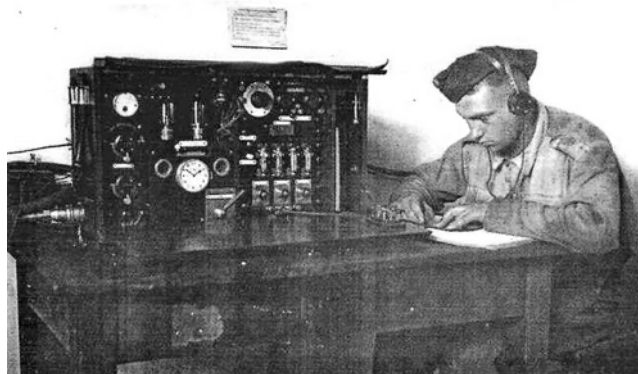
Operator of a stationary RKA wireless station. Note the two type MT5 valves in the transmitter.
